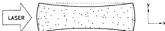
Figure 5. Visualization of the effect of light-induced pressure anisotropy in a cell having flexible walls (see equation (6)).
